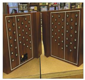
The stop jams refinished and loaded with new felt and hardware to accept the new stops.
